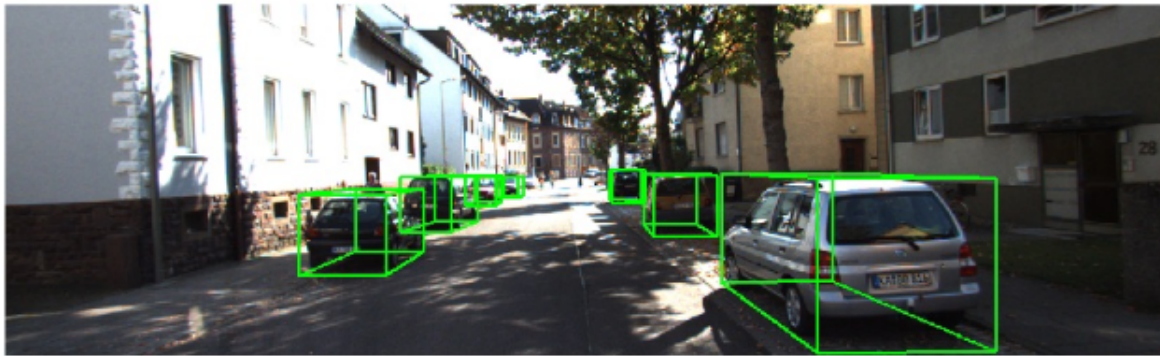
Figure 1 – Example of 3D object detection in an urban scenario, highlighting how objects are marked. Adapted from (SINDAGI; ZHOU; TUZEL, 2019).
