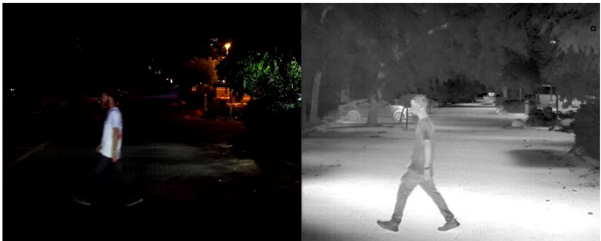
Figure 4 – Comparison of images obtained from the RGB camera (left) and thermal camera (right) taken from the ForesightAuto page. (DANZIGER, 2020).
